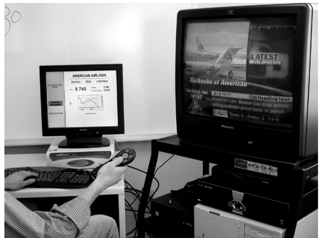
Figure 1. A television viewer receives information on a computer (left) after using the remote control to signal interest in the story currently on the television.
